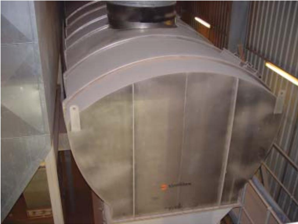
*The gas-fired Ventilex fluidized-bed dryer*
