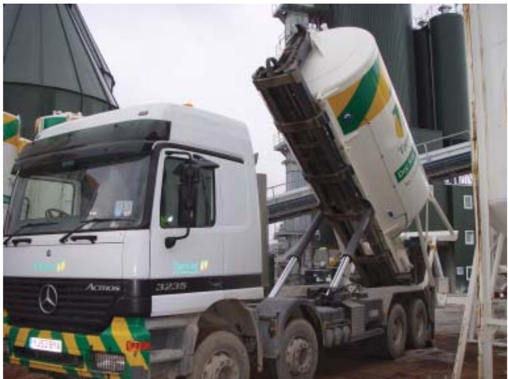
A mobile DSM silo being loaded for delivery to site
